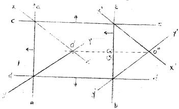
probable location for the three lines b-b, c-c and d-d, while O at a point midway between O' and O" is the most probable position of the four lines, assuming that all sights have the same value.
