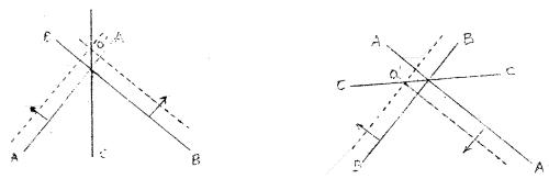
error will effect each Summer line, and remembering that this error will affect each line in the same direction, either towards or away from both objects observed. The intersection of these dotted lines is at O', which shows the line must pass through O' and be the line C-C in both cases.
