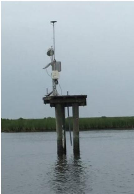
Figure 2: Figure showing GNSS setup at Delacroix station.
